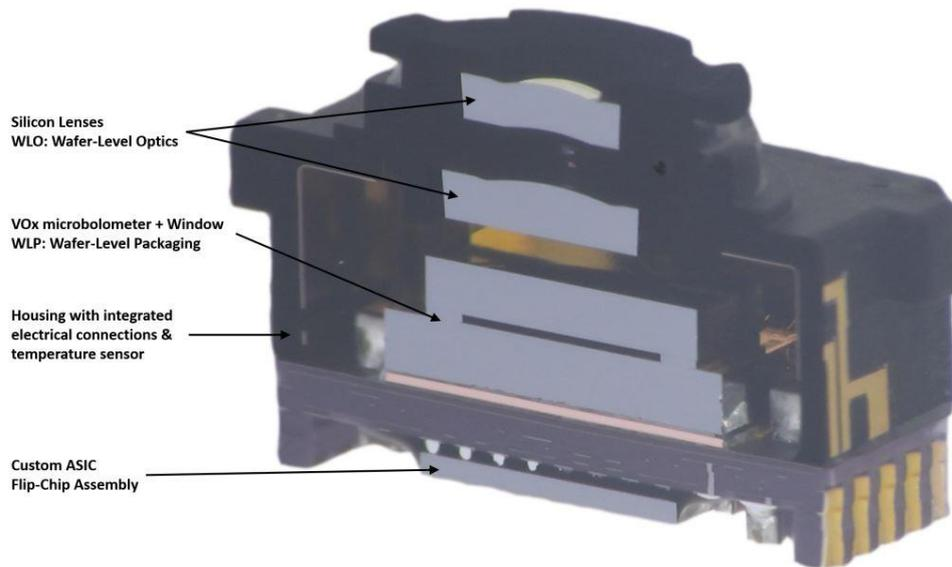
*LEPTON Infrared Camera Module Cross-Section*
