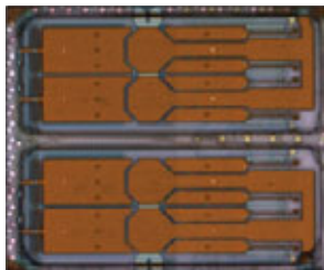
4 Single Capacitors (Courtesy of System Plus Consulting)
