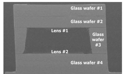
OVM7692 Wafer-level optics cross-section
