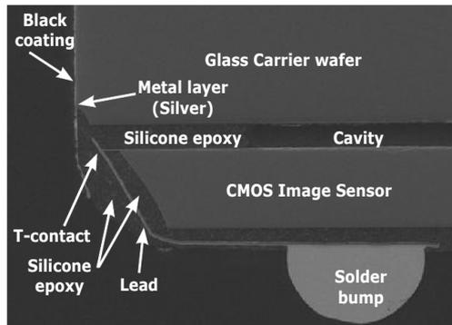
OVM7692 ShellCase CIS WLP cross-section (Courtesy of System Plus Consulting)
