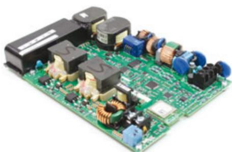
The Power-One microinverter's electronic board (Courtesy of System Plus Consulting)
