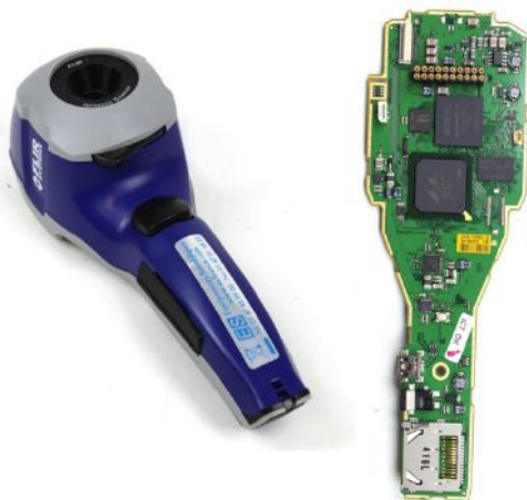
i7 Camera teardown (Courtesy of System Plus Consulting)
