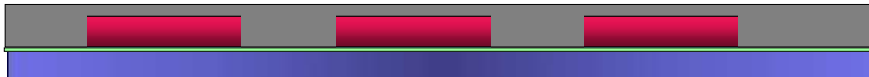
5) Grinding of the epoxy resin (to release the stress difference between both sides so as to avoid wafer warping?)
